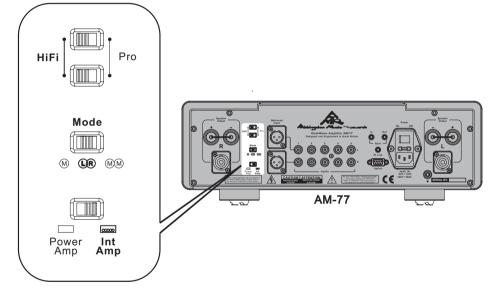
For the majority of sources, the HiFi/Pro switch (R3) is best left in the 'HiFi' position. However, if the source has a pro-audio style transformer balanced output, the HiFi/Pro switch needs to be set to 'Pro'.
